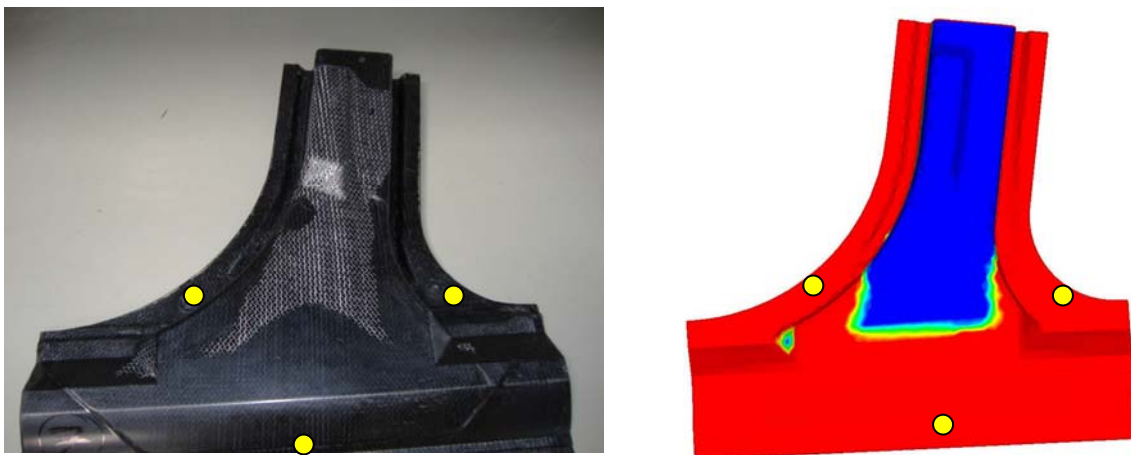
Fig. 7 Filling profile of the carbon preform industrial part after 67 s.
